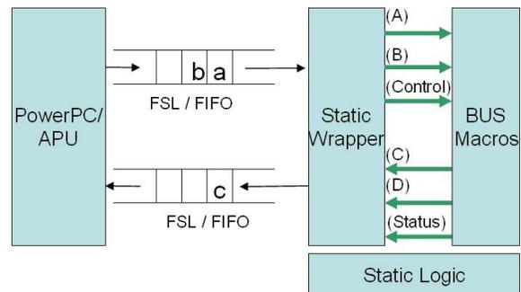
Figure 5. Data flow using FSL from the APU to the static wrapper
