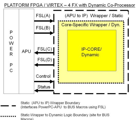
**Figure 1. System Architecture of the dynamic co-processor system**
