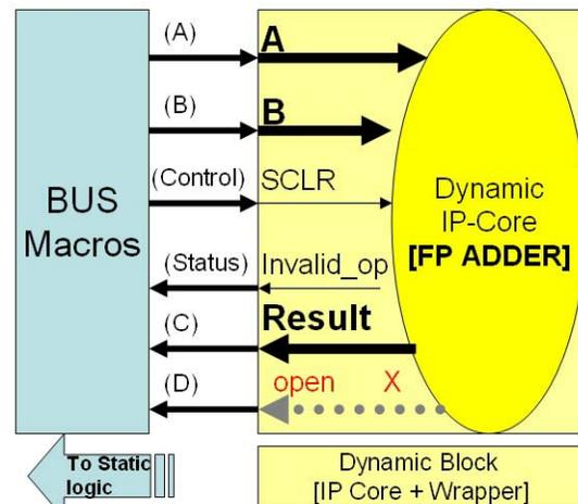
Figure 6. The dynamic block consisting of the dynamic wrapper around its accompanying dynamic IP Core
