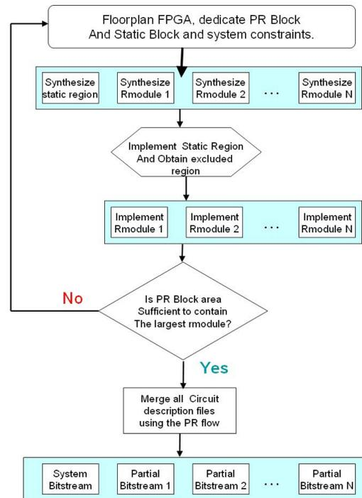
**Figure 8. The Partial Reconfiguration Flow for FPGA**
