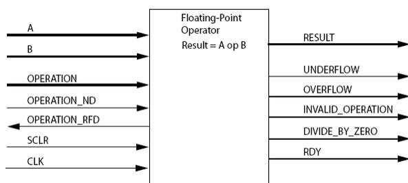
**Figure 2. An example Floating Point IP Core**
