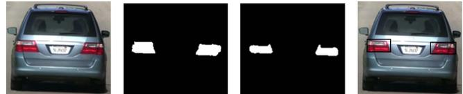
Fig. 6. Tail light detection
