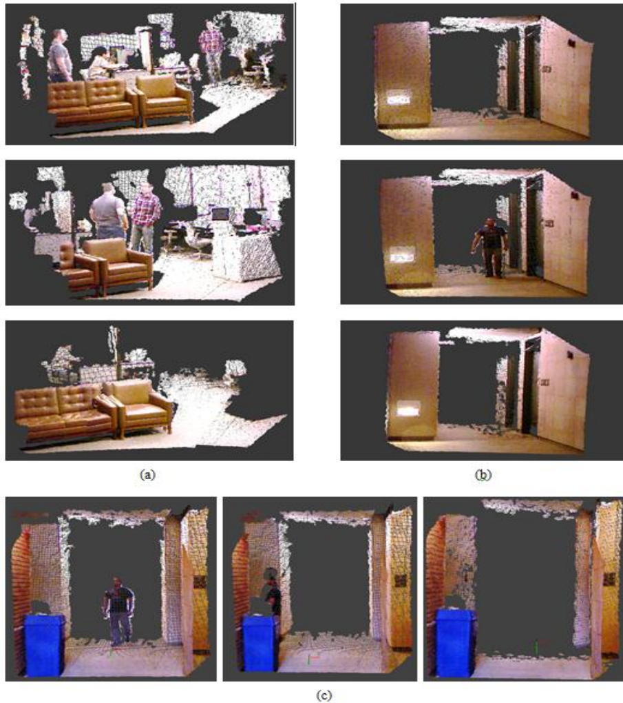
Fig. 5. Example results. (a) office scene with three people (two walking, one sitting). The top two frames from columns (a) and (b) were merged together to produce the bottom point cloud. (b) corridor scene where the person just entered the corridor through a door on the right. (c) a walking person changing direction.
