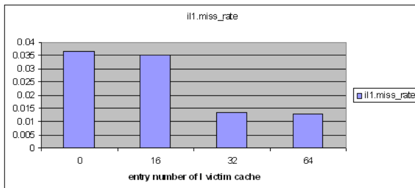
Figure 3: Miss rate at level-1 I-cache is reduced with increased victim cache attached
