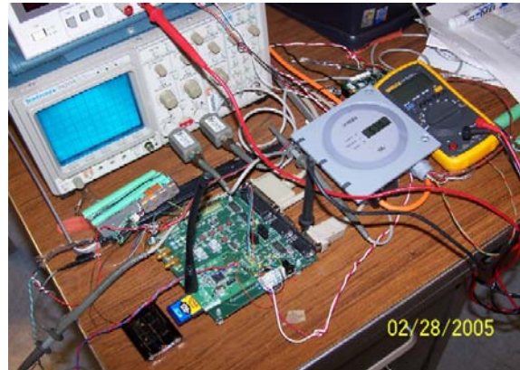
Figure 7. The RISE node interfaced with the Vaisala GMT 220 CO 2 sensor.
