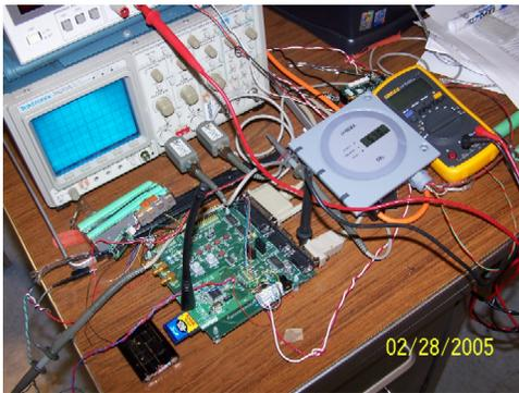
Figure 2. The RISE node interfaced with the sensors and the evaluation testbed.
