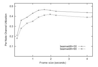
Fig. 9. Per node CUR achieved vs. frame size in random mobile topology with speed = 2m/s.
