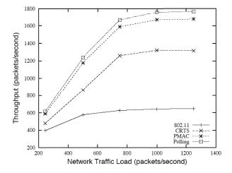
Fig. 4. Total network throughput vs. network traffic load in stationary random topology.
