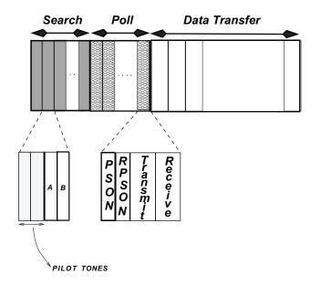
Fig. 1. Frame structure in PMAC.
