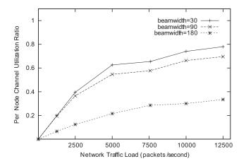
Fig. 6. Per node channel utilization ratio vs. network traffic load in stationary random topology.
